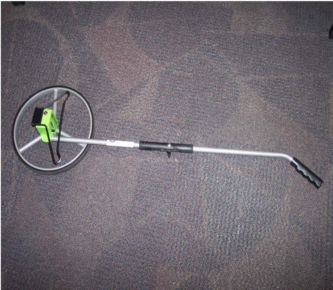
Figure 3-11: Walking measuring wheel
